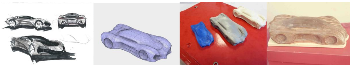
Figure 1. The concept car project, from left to right: sketch, virtual model, 3 printed out, wooden rapid prototype
