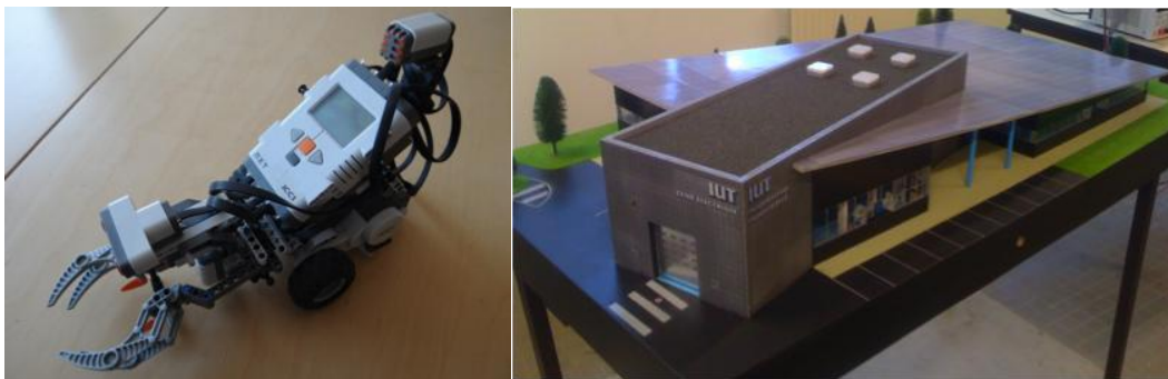
Figure 3: Left, a rover in Lego bricks moving in a maze ; Right, a building mock up equipped of sensors to be programmed
