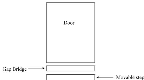
**Fig. 2** The passenger access system
