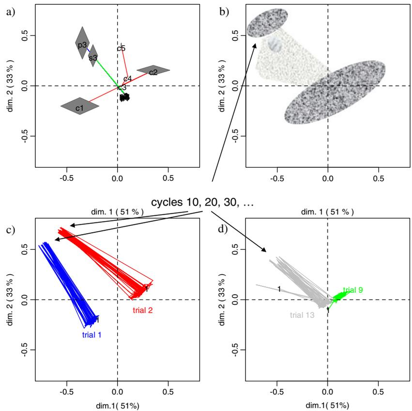
MCA also allows to highlight outliers. This is the case of the first cycle of trial 13 during which the set of factor levels do not permit the closing of the door within 3.5 s. In fact, the door control unit (DCU) operations are based on a learning feedback from the previous cycles. For this reason, only the first cycle is mainly impacted (Fig. 6d).
