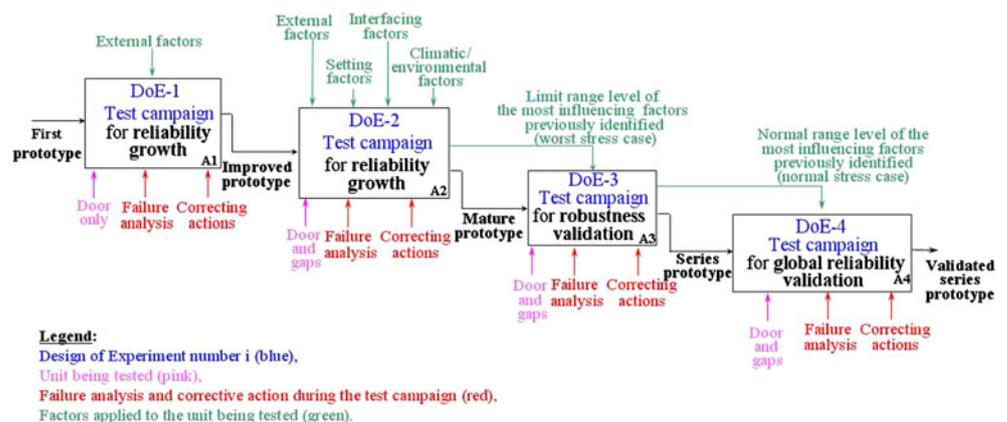
this study. It would be too restrictive and too expensive to provide a set of interchangeable structures to represent all the possible configurations. We therefore chose a “worst case” in terms of manufacturing tolerances for the vehicle structure.
