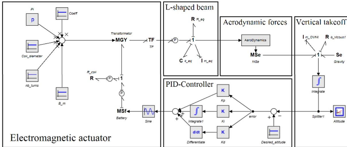
Fig. 8. Bond Graph model of closed loop fly.
