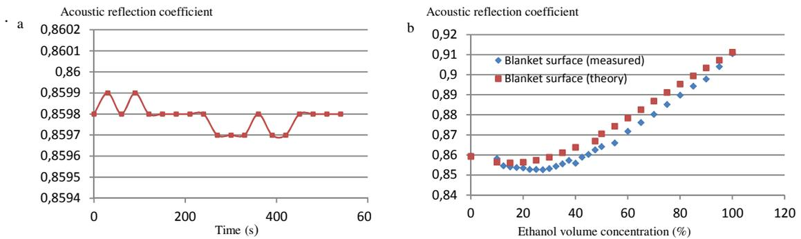
**Fig. 1.** Acoustic reflection coefficient  $|R|_{\text{norm}}$ : a) measured for water (21°C) as a function of time ; b) calculated and measured in ethanol/water mixtures as a function of Ethanol Volume Concentration .
