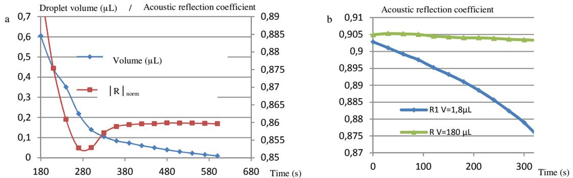
**Fig. 3.** Evolution of the acoustic reflection coefficient at the interface liquid/silicon: a) 1  $\mu\text{L}$  droplet of pure ethanol at 99,9% (the evolution of the volume is also given) ; b) comparison between a 1 $\mu\text{L}$  droplet and a bigger volume of 180  $\mu\text{L}$ .
