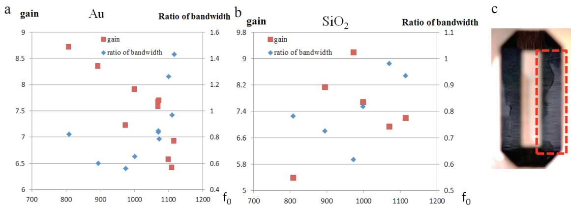
**Fig. 3.** Gain and bandwidth ratio comparison: a) with 800 nm gold layer introduction; b) with 3.8 $\mu$ m SiO<sub>2</sub> layer; c) SiO<sub>2</sub> film partially lift-off.  $f_0$  is the experimental central frequency of transducer.
