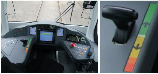
(a) Tram cabin control (b) Haptic manipulator
