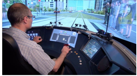
Fig. 3. PSCHITT-rail tram simulator.
