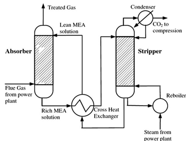
Fig. 1 Schematic diagram of PCC process (Lawal *et al.* 2010)
