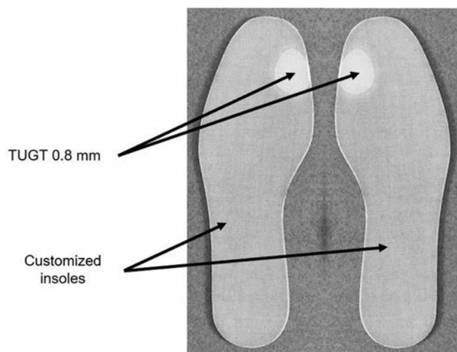
Figure 3. Example of customised postural insoles. The insoles were made of a rigid polyester resin. The hardness was 60 Shore A, and the density was 250 kg/m<sup>3</sup>. They had a thickness of 1 mm and their size of the insoles is adapted to the size of the subject's feet. TUGT are inserted in both insoles and positioned exactly under the great toes. TUGT: Thickness under Great Toe.
