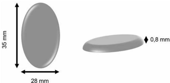
Figure 1. TUGT were made of a rigid polyester resin and with an ovular form. The hardness was 60 Shore A, and the density was 250 kg/m<sup>3</sup>. They had a width of 28 mm, a length of 35 mm and a thick of 0.8 mm. TUGT were placed under the plantar surface of great toe of both feet. TUGT: Thickness under Great Toe.
