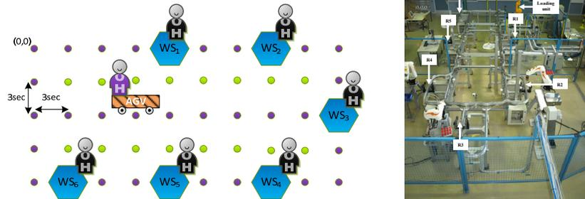
Fig. 5. Cell configuration test scenario (on the right side the real AIP cell).
