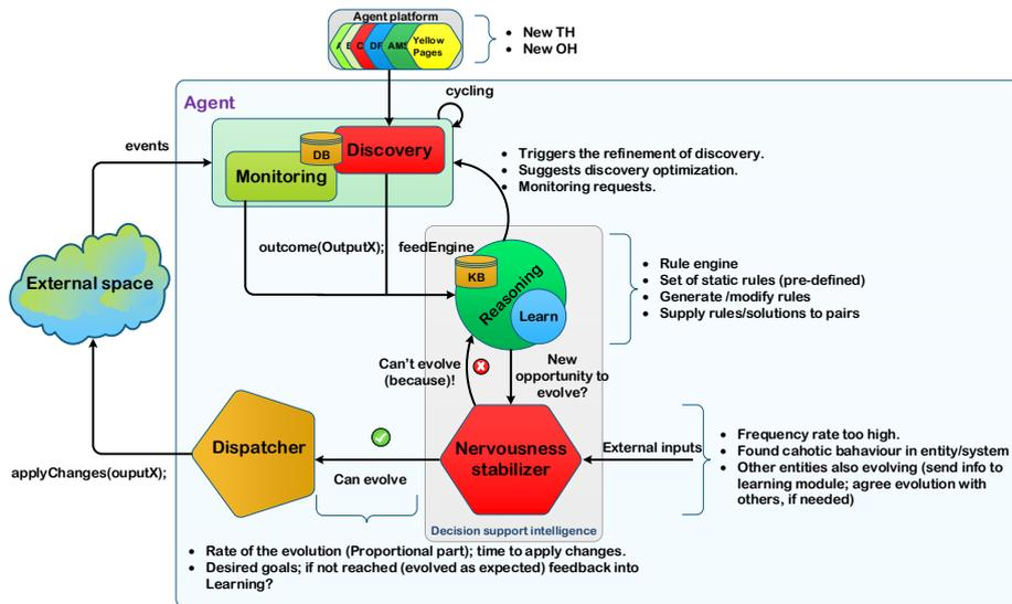
Fig. 4. Model to support the self-organization mechanisms
