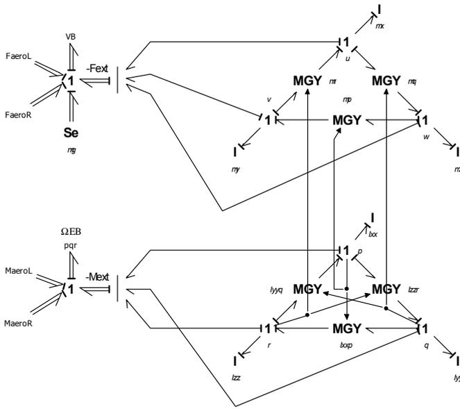
Fig. 3. Bond graph representation of Newton-Euler equations.
