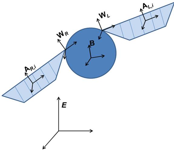
Fig. 1. Flapping wing MAV schematic with reference frames.
