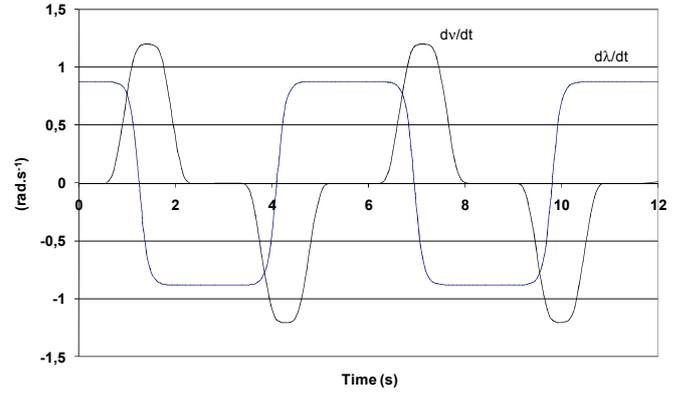
Fig. 4. Flapping and pitch angular velocities.
