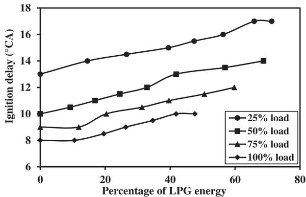
Fig. 11 Variation of ignition delay with LPG-RSO dual-fuel engine operation at different loads
