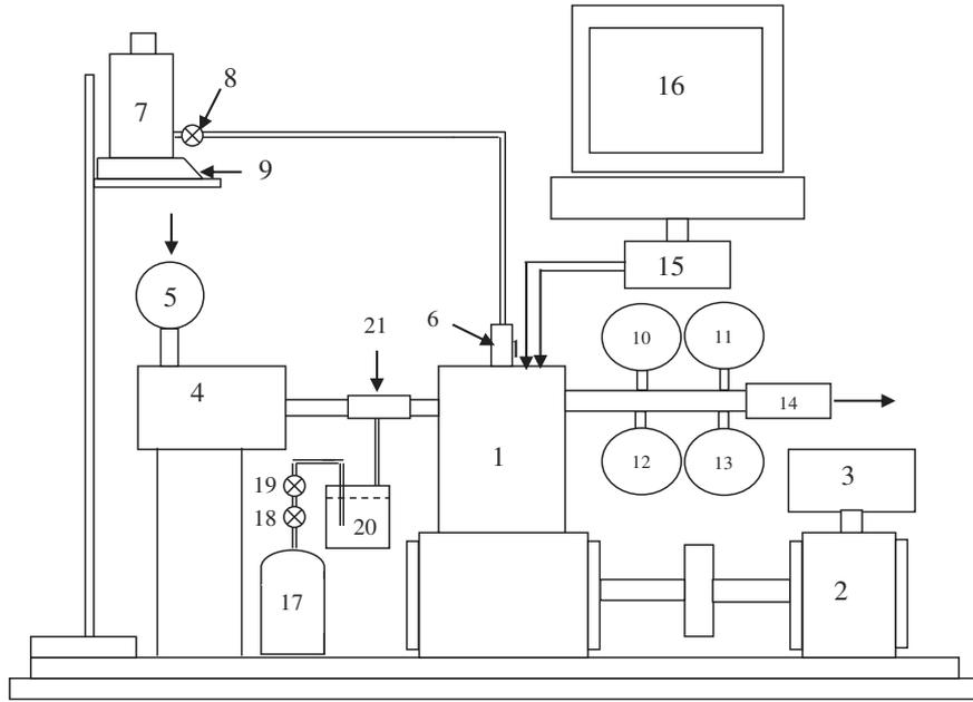
**Fig. 1 Schematic of the experimental setup: 1, engine; 2, dynamometer; 3, control panel; 4, air tank; 5, air flow meter; 6, injector; 7, fuel tank; 8, fuel valve; 9, balance; 10, smoke pump; 11, FID; 12, CO analyzer; 13, NO analyzer; 14, silencer; 15, charge amplifier; 16, computer; 17, LPG cylinder; 18, pressure regulator; 19, control valve; 20, flame trap; 21, LPG injector**
