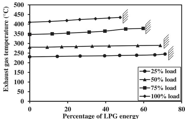
Fig. 3 Variation of exhaust gas temperature with LPG-RSO dual-fuel engine operation at different loads
