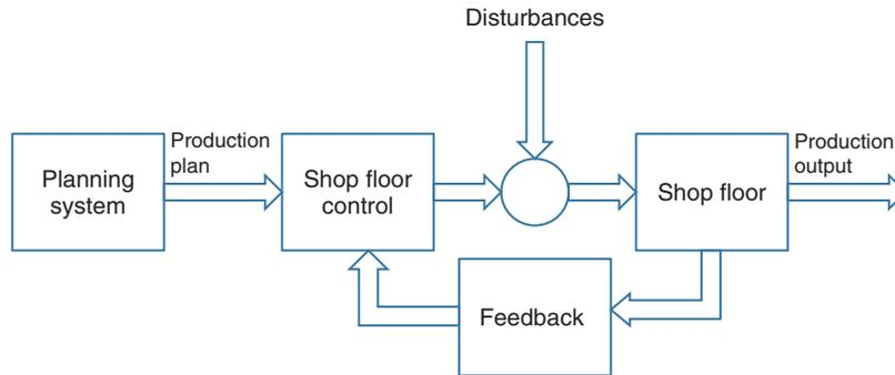
**Figure 1.** Functioning of shop-floor control.
