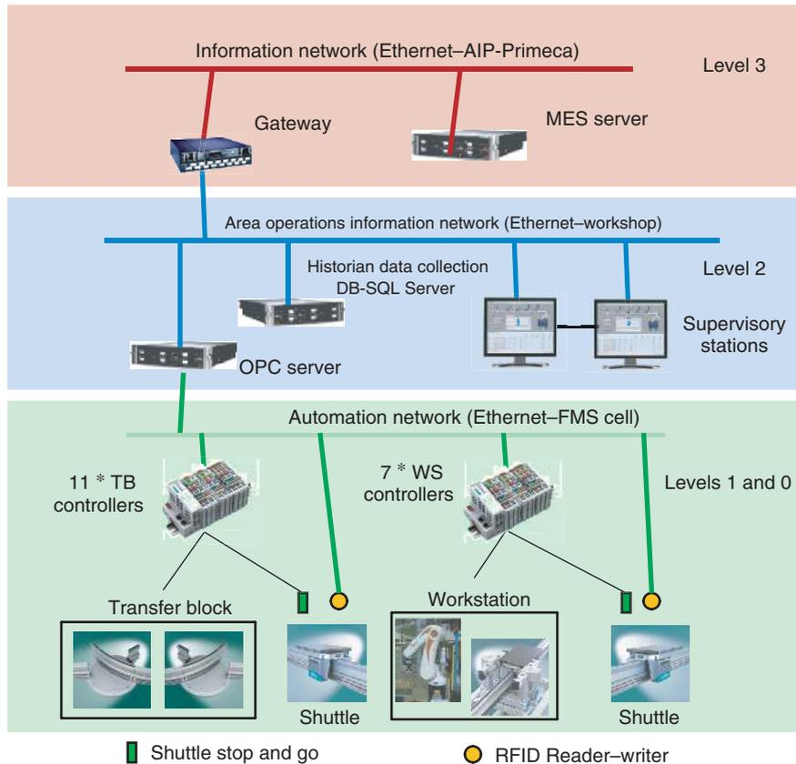
**Figure 5.** Modern SFC architecture of the AIP cell.
