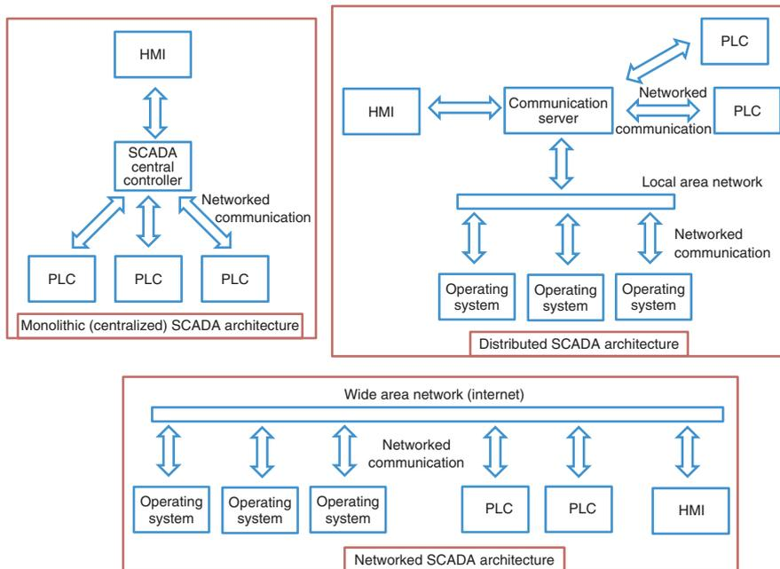
**Figure 2.** Typical SCADA architectures. *Source:* Adapted from NCS [1].
