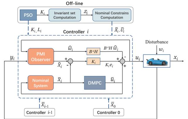
Fig. 3. Structure of the proposed integrated control scheme.
