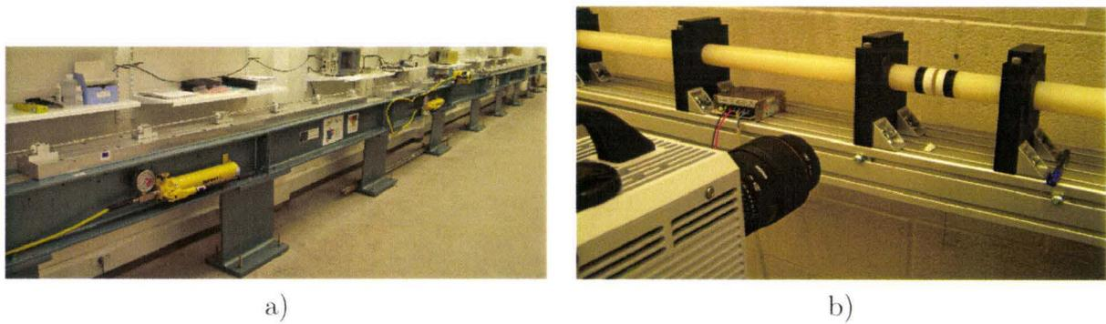
Figure 2.7: a) pre-stressed tensile and b) visco-elastic compressive Hopkinson bars.
