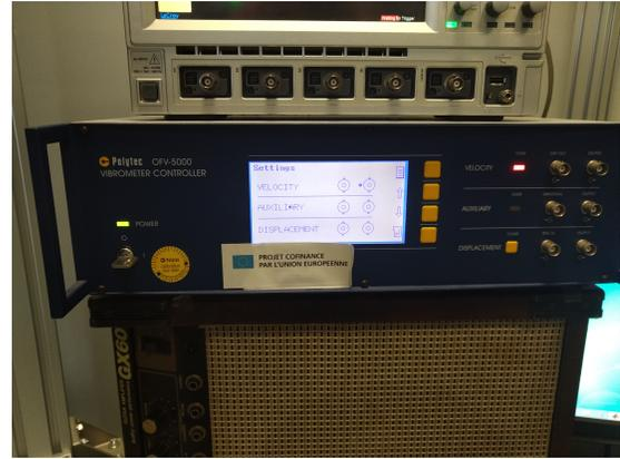
(b) Laser vibrometer controller.
